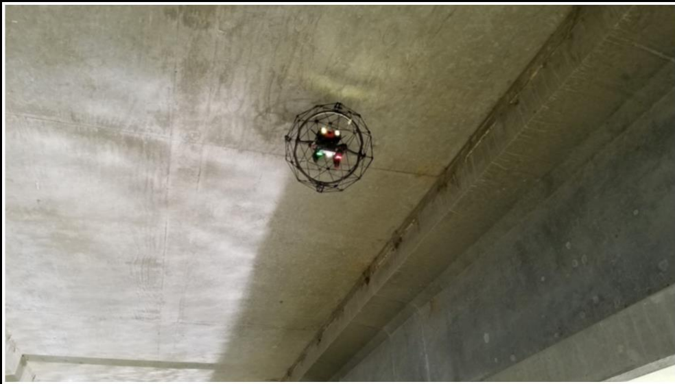
Elios UAS in contact with bridge soffit and abutment
